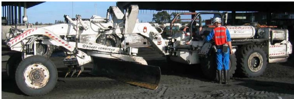
Figure 3-9: Underground grader [WINKEL]
